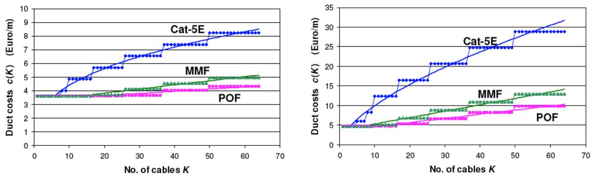
Figure 3: Costs of installed ducts; on-the-wall mounted (l.) and buried (r.) (from [9])
