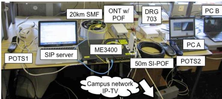
(c) Trial setup with the POF PON located on table to the right
